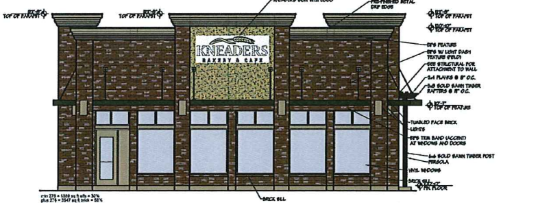
FRONT EXTERIOR ELEVATIONS 1 1/4" = 1'-0"
