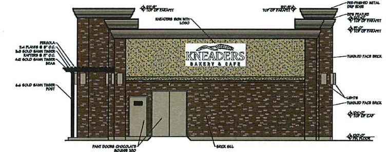
BACK EXTERIOR ELEVATIONS 3 1/4" = 1'-0"
