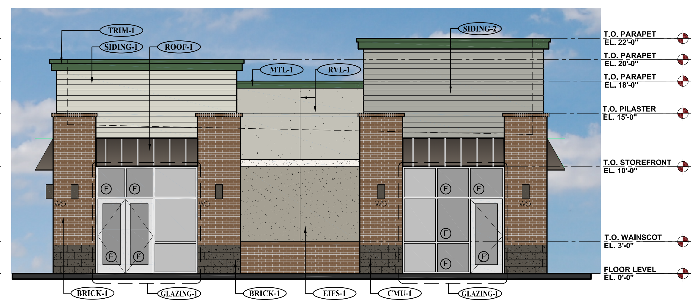
3 A-1 PROPOSED WEST ELEVATION (RIGHT SIDE) SCALE: 3/16" = 1'-0"
