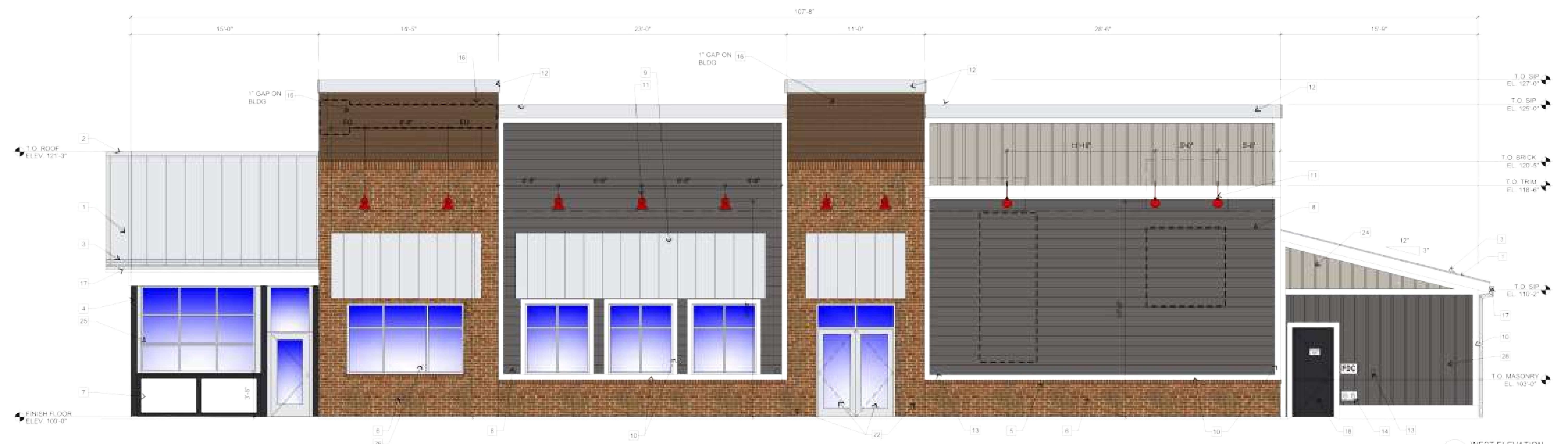
1 WEST ELEVATION SCALE: 1/4" = 1'-0"
