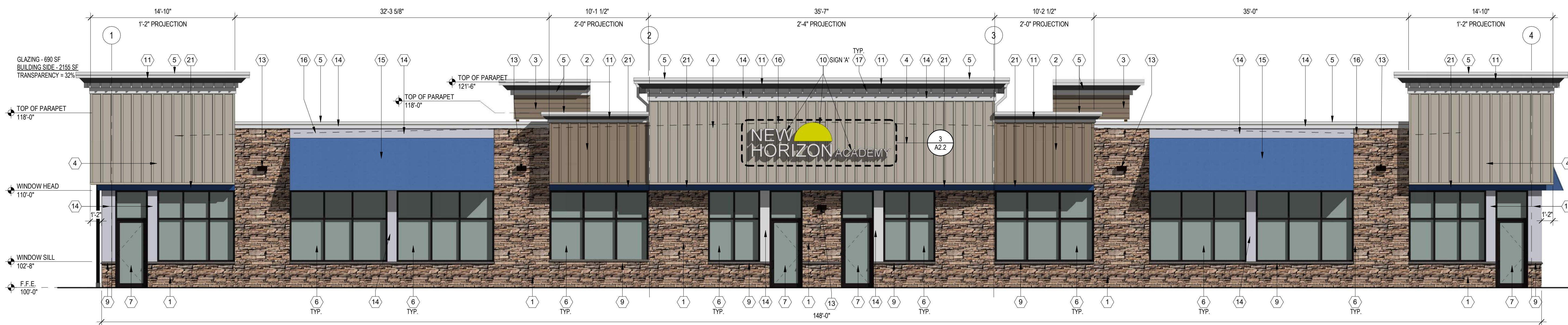
1 EAST ELEVATION SCALE: 3/16" = 1'-0" 0' 2' 6' 12' 21'-4"
