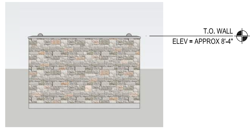
9 ENCLOSURE LOTS 1 & 2 REAR ELEVATION NTS
