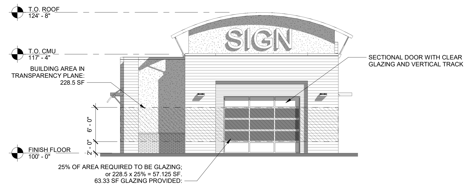
2 EXIT/SOUTH ELEVATION TRANSPARENCY DIAGRAM 1/8" = 1'-0"
