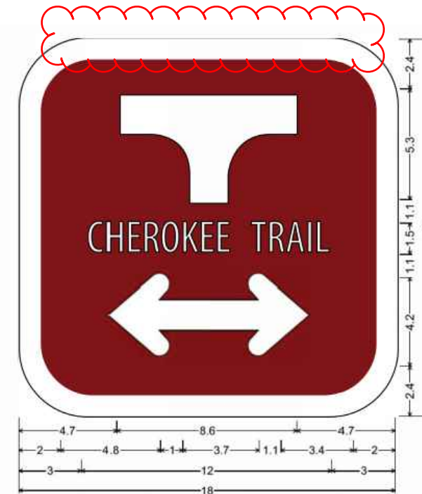
3.0" Radius, 1.0" Border, White on Brown; sign int shape; "CHERRY CREEK TRAIL" B specified length; Double Headed Arrow Custom - 12.0" 0";
