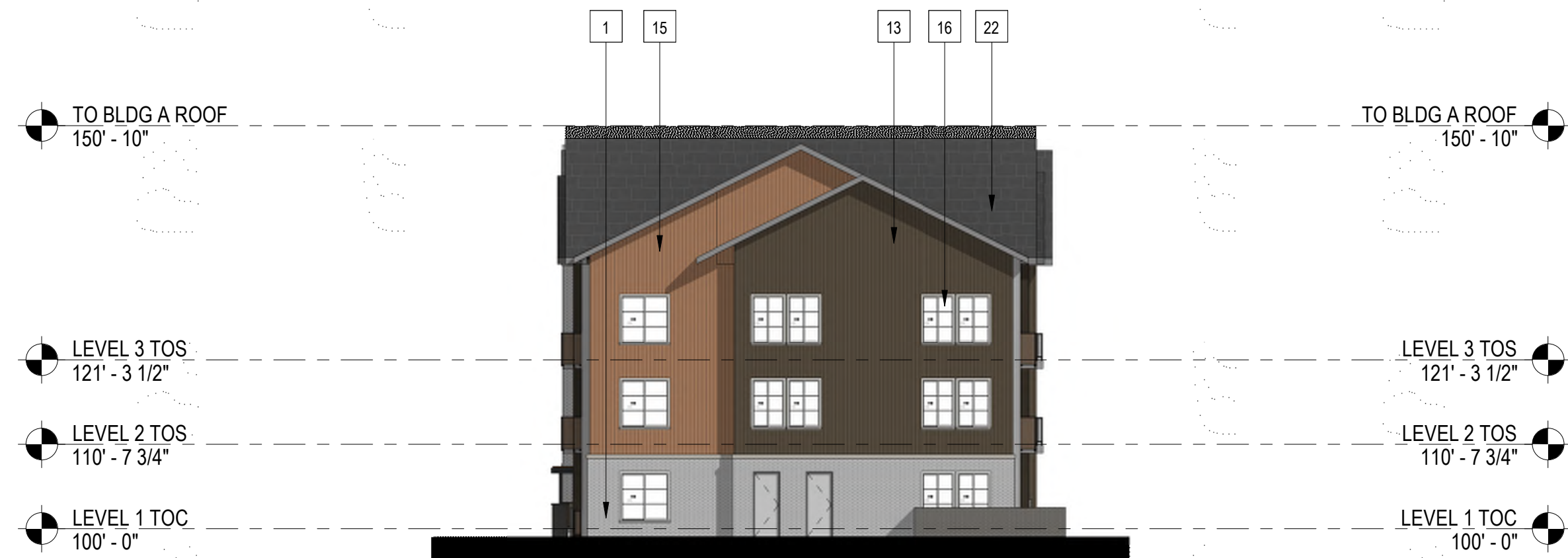
3 BUILDING C - ELEVATION 1/16" = 1'-0"
