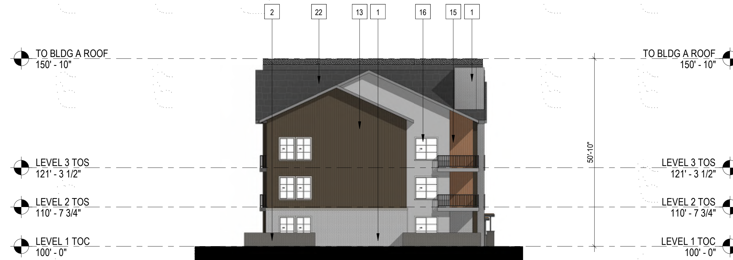
4 BUILDING C - ELEVATION 1/16" = 1'-0"
