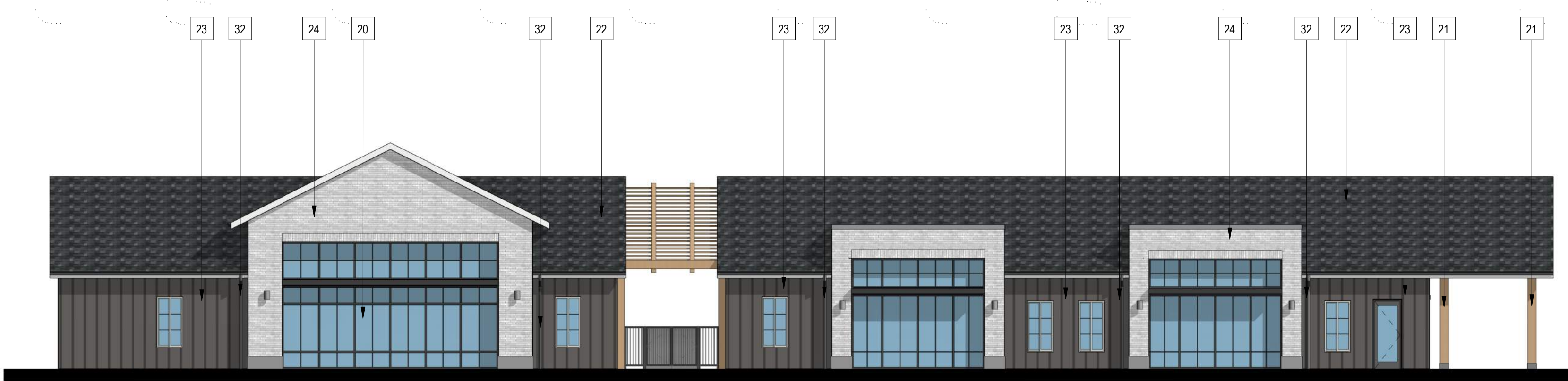
FRONT ELEVATION Note: Trim around windows shall be minimum of three and one-half (3-1/2) inches wide, and trim around doors shall be a minimum of (2) inches wide.
