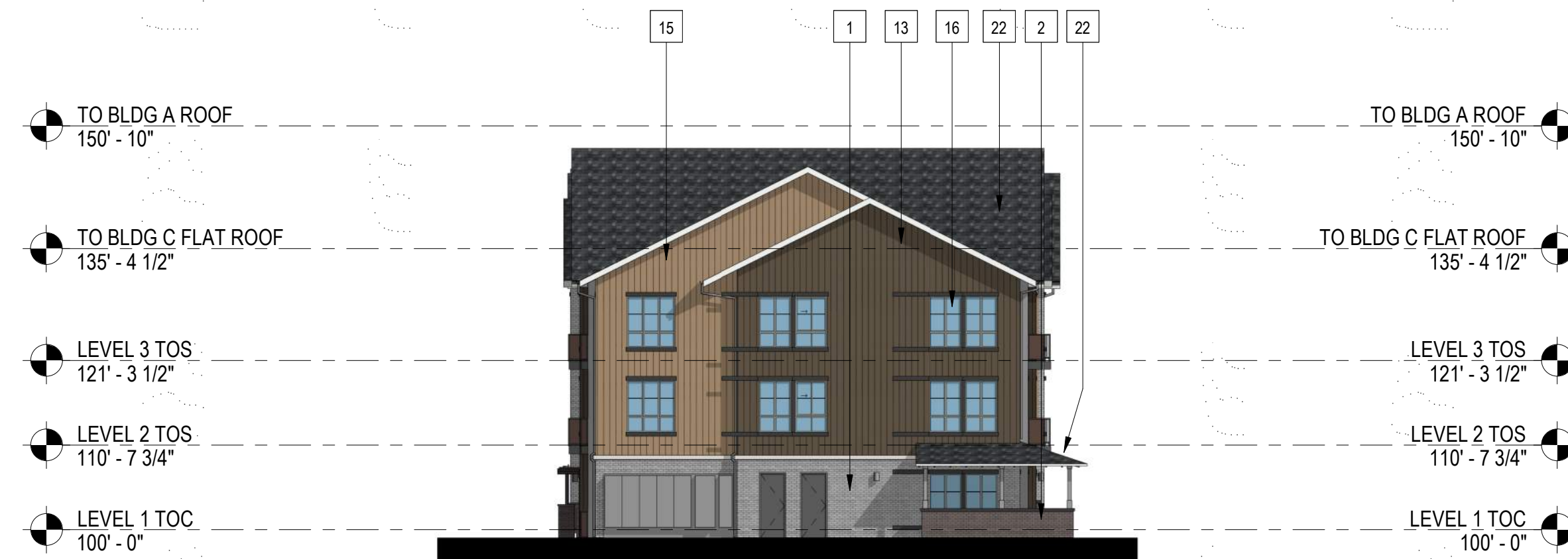
3 BUILDING C - SIDE ELEVATION 1/16" = 1'-0"
