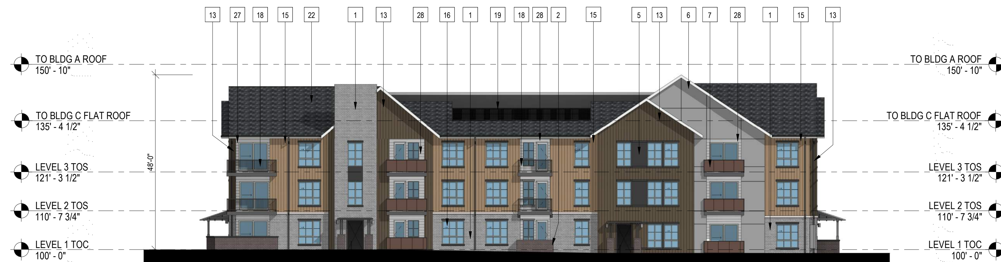
1 BUILDING C - FRONT ELEVATION 1/16" = 1'-0"
