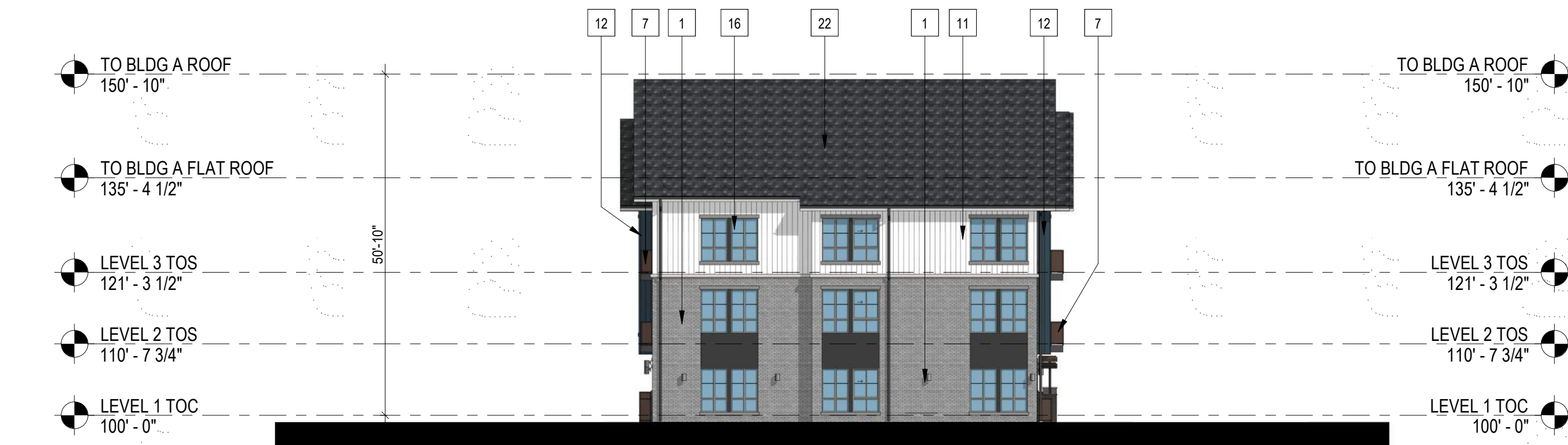
4 BUILDING A - SIDE ELEVATION 1/16" = 1'-0"
