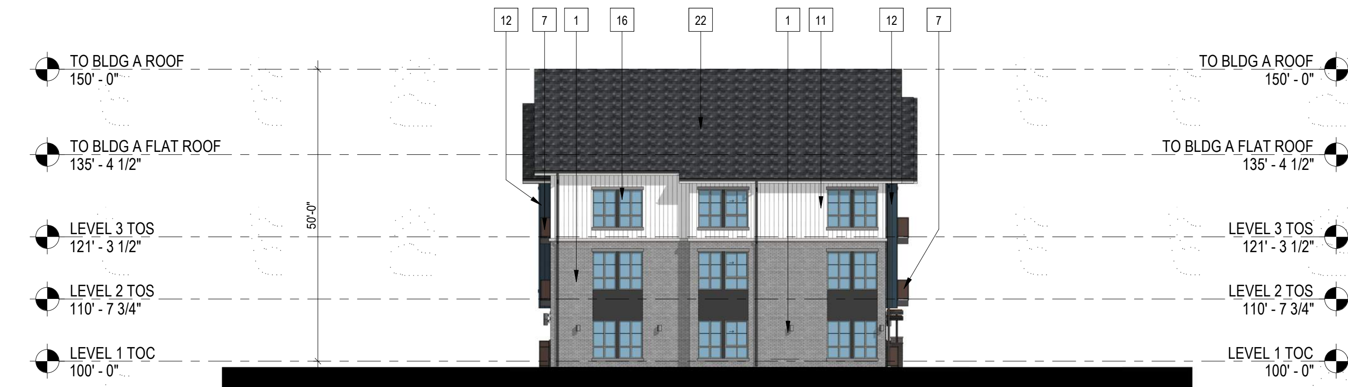
4 BUILDING A - SIDE ELEVATION 1/16" = 1'-0"
