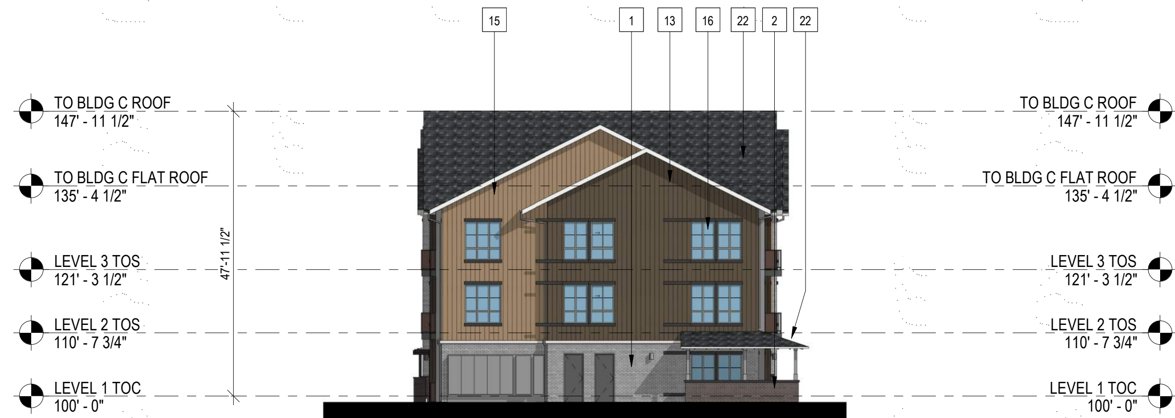
3 BUILDING C - SIDE ELEVATION 1/16" = 1'-0"
