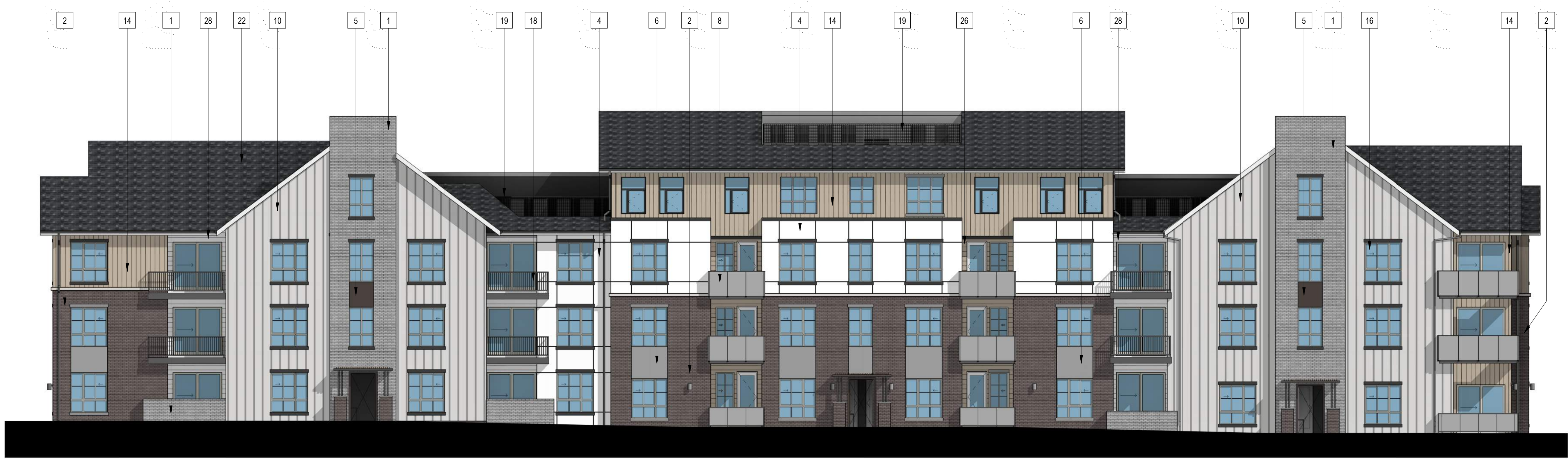
FRONT ELEVATION Note: Trim around windows shall be minimum of three and one-half (3-1/2) inches wide, and trim around doors shall be a minimum of (2) inches wide.
