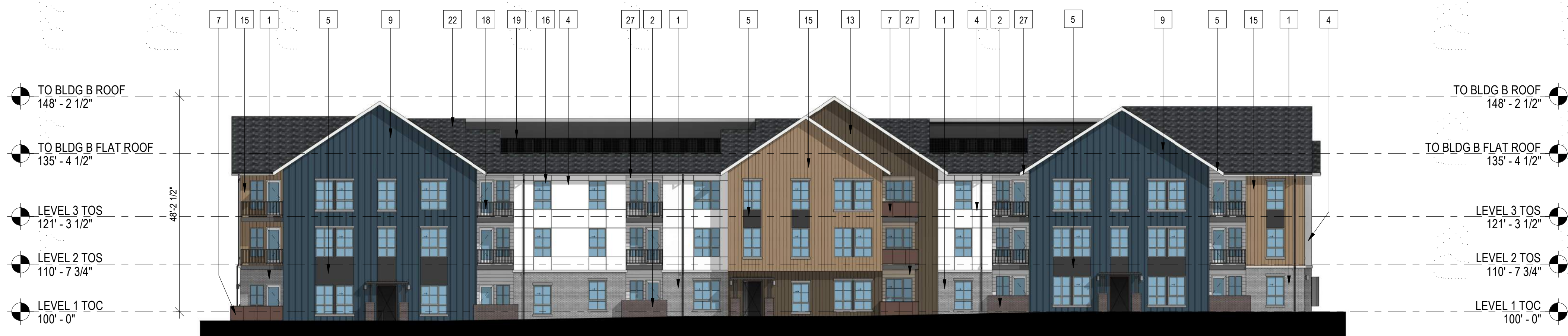
2 BUILDING B - REAR ELEVATION 1/16" = 1'-0"
