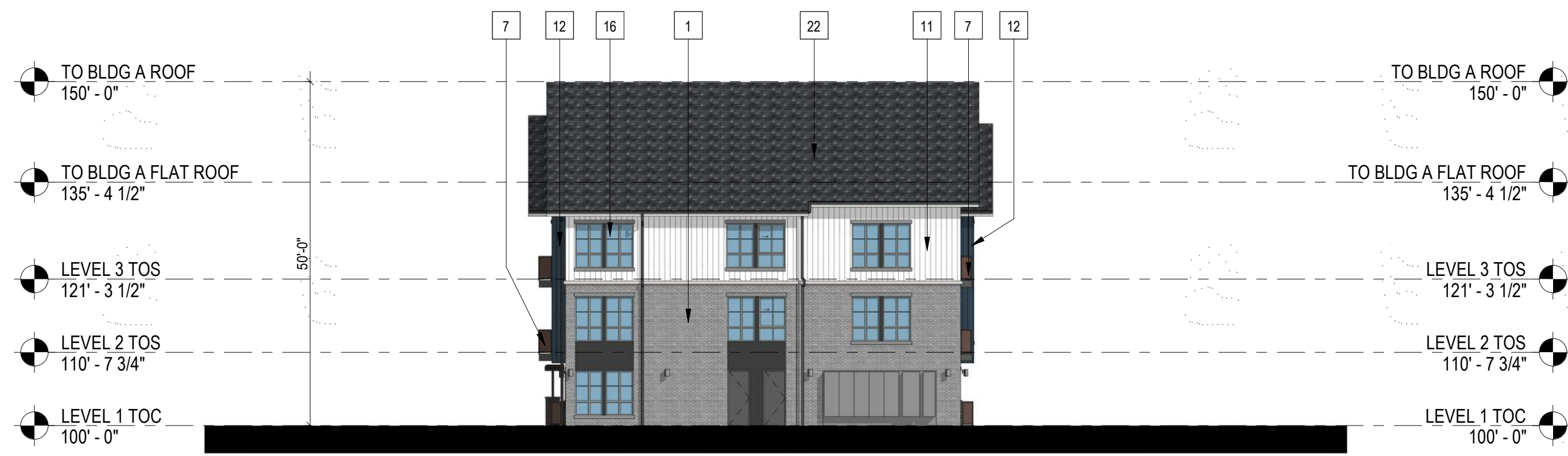
3 BUILDING A - SIDE ELEVATION 1/16" = 1'-0"
