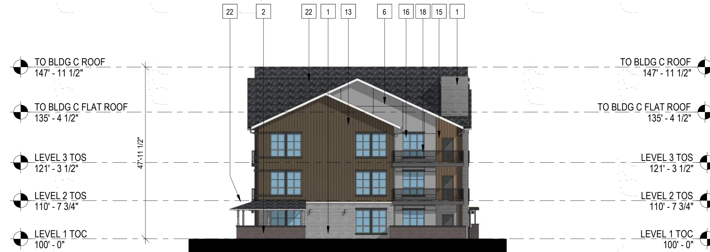
4 BUILDING C - SIDE ELEVATION 1/16" = 1'-0"
