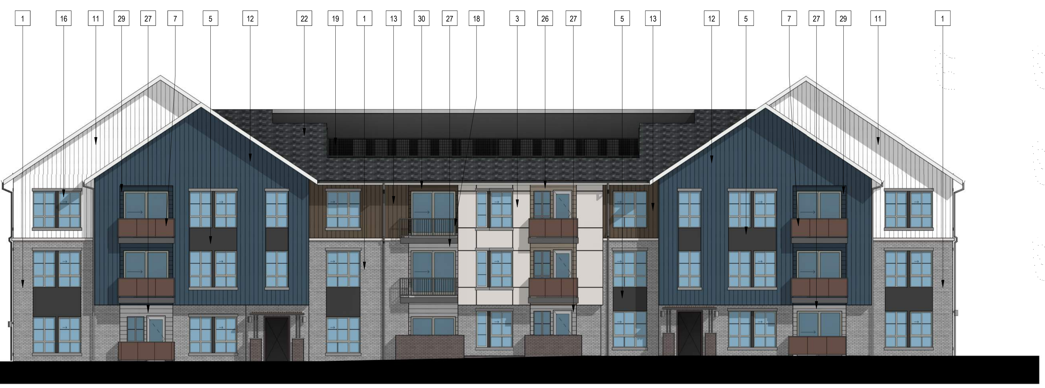
FRONT ELEVATION Note: Trim around windows shall be minimum of three and one-half (3-1/2) inches wide, and trim around doors shall be a minimum of (2) inches wide.
