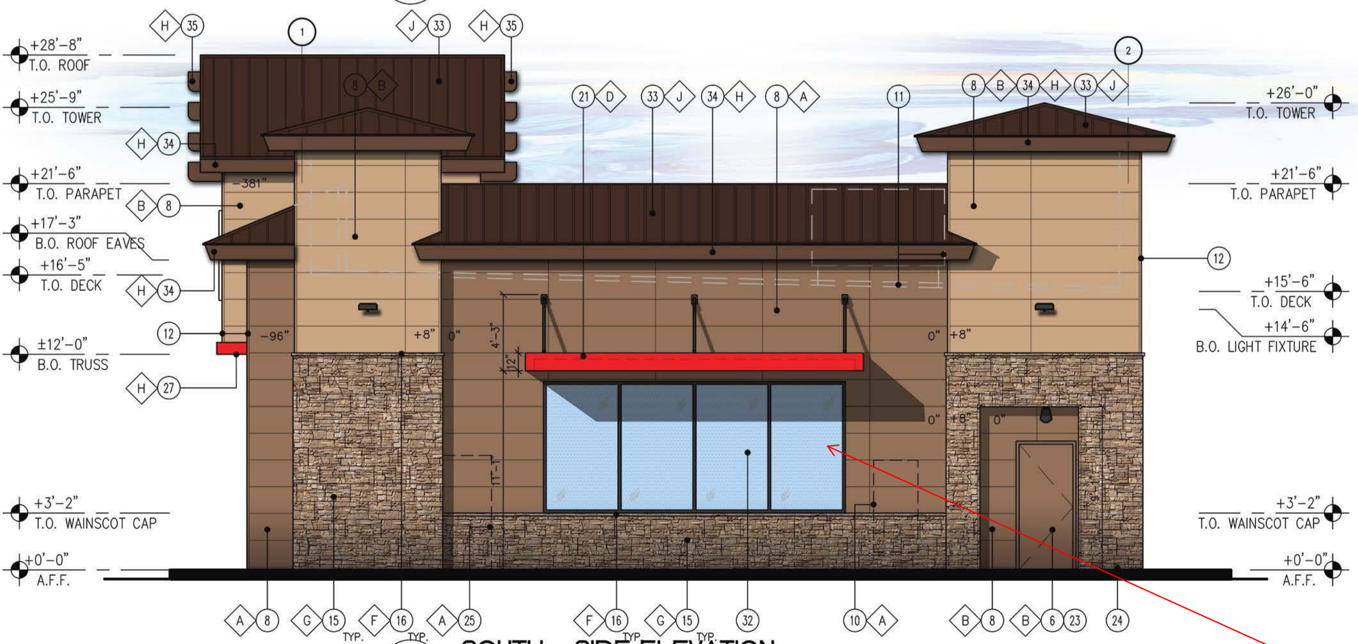
3 SOUTH - SIDE ELEVATION SCALE: 3/16" = 1'-0"
