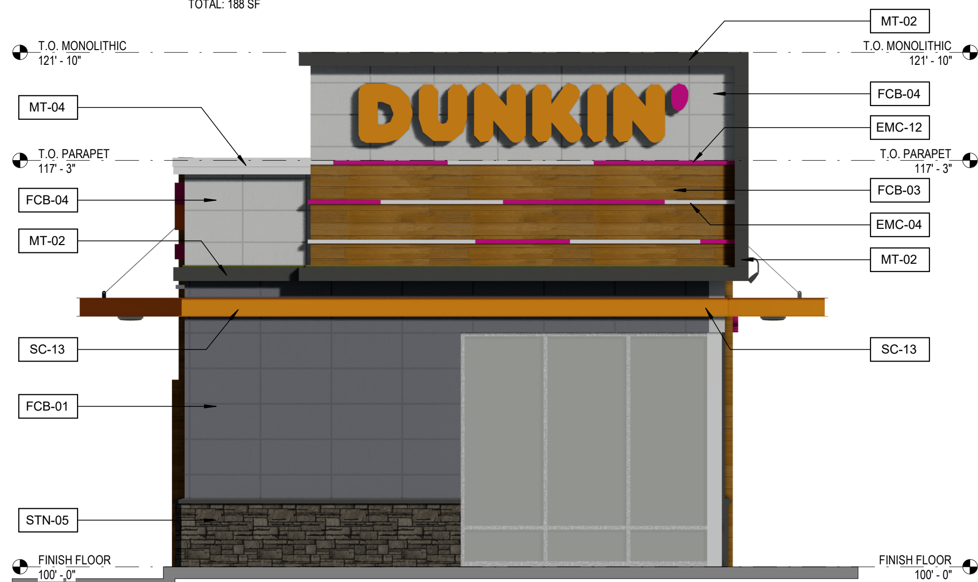
2 EXTERIOR ELEVATION - FRONT SCALE: 1/4" = 1'-0"
