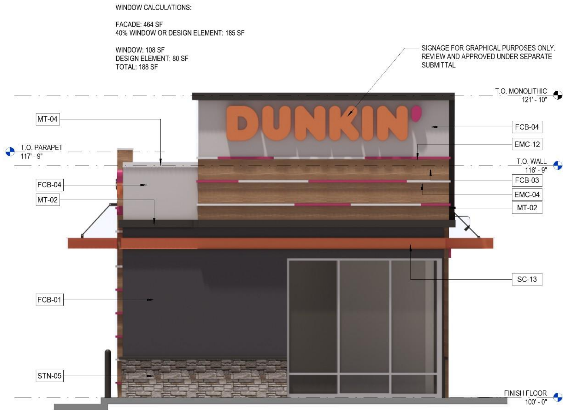
2 EXTERIOR ELEVATION - FRONT (WEST) SCALE: 1/4" = 1'-0"
