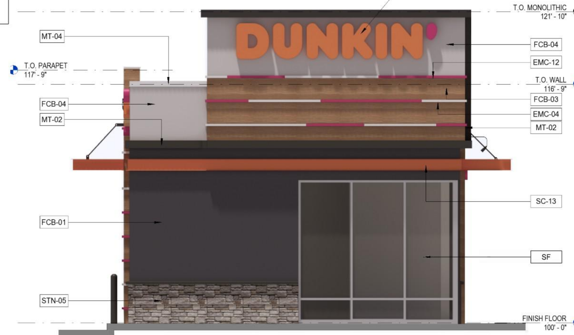
2 EXTERIOR ELEVATION - FRONT (WEST)
