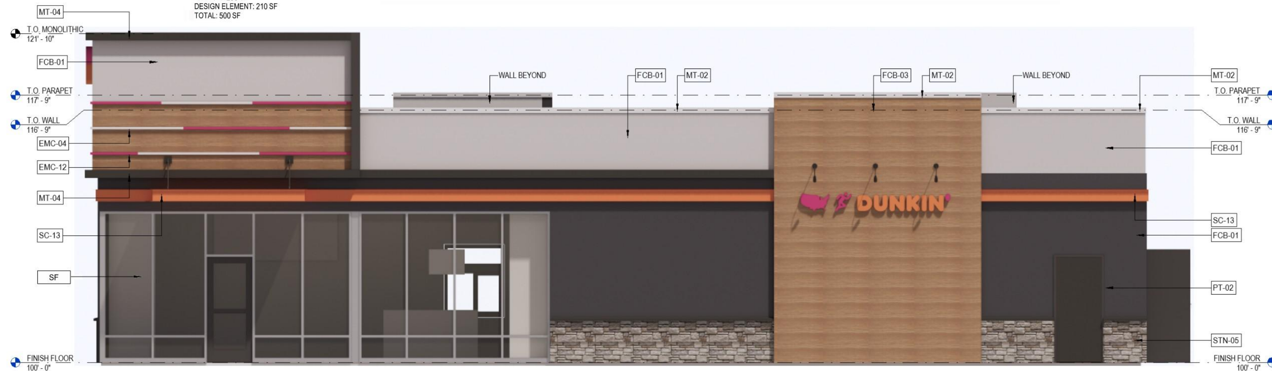
1 EXTERIOR ELEVATION - RIGHT SIDE (SOUTH) SCALE: 1/4" = 1'-0"
