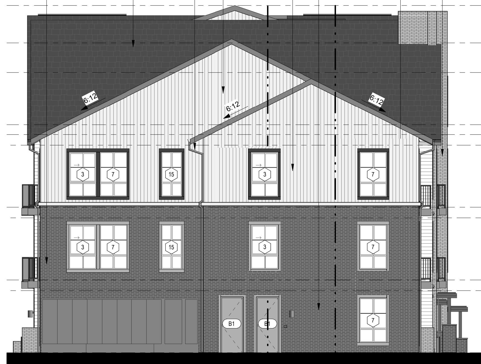
New proposed elevations for Building 1 and 4 only. Remove two rows of windows
