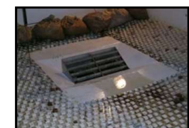
CDOT Type D Inlet Parallel (30° Incline & Depressed)
