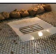
CDOT Type D Inlet Parallel (10° Incline & Depressed)
