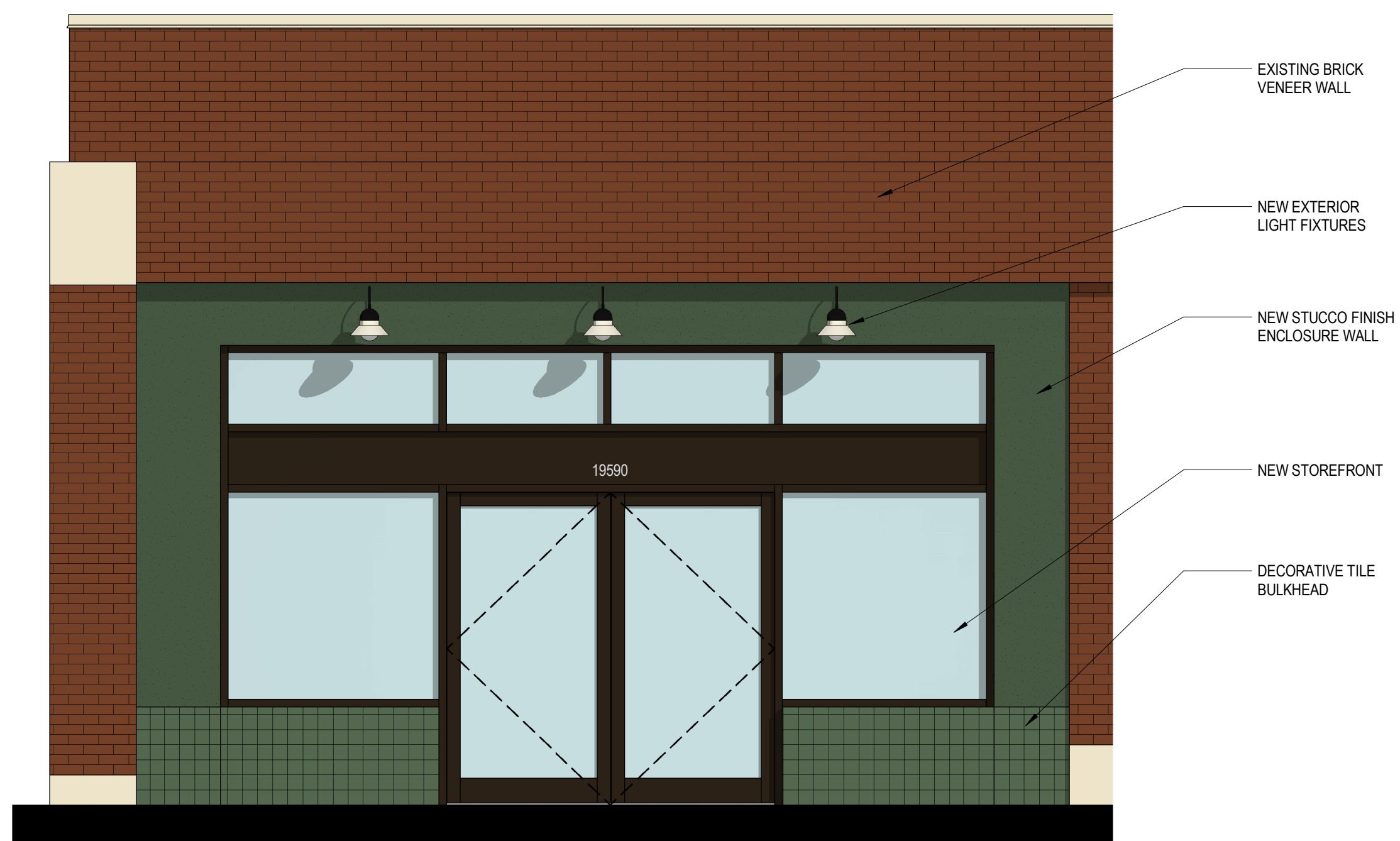
2 PROPOSED INFILL WALL ELEVATION SCALE: 3/8" = 1'-0"
