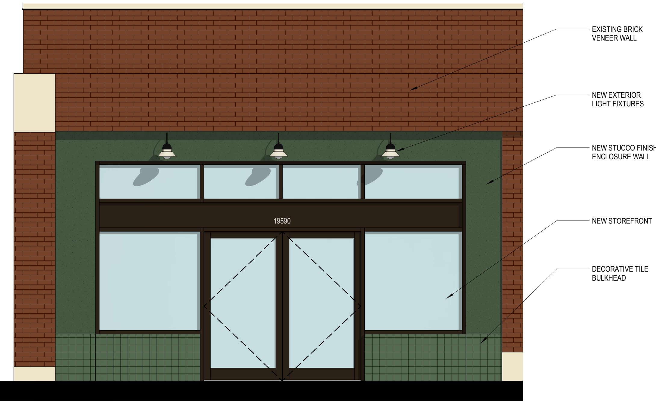
2 PROPOSED INFILL WALL ELEVATION SCALE: 3/8" = 1'-0"
