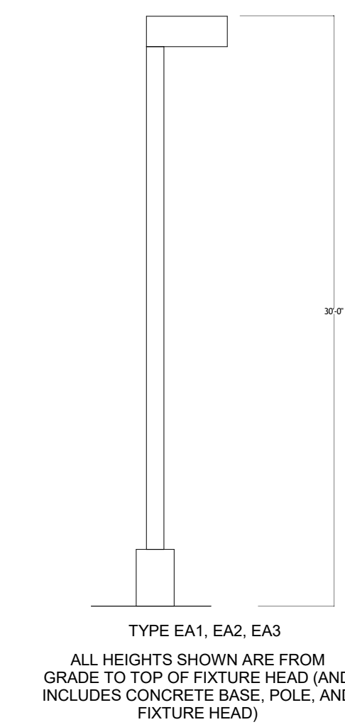
TYPE EA1, EA2, EA3 ALL HEIGHTS SHOWN ARE FROM GRADE TO TOP OF FIXTURE HEAD (AND INCLUDES CONCRETE BASE, POLE, AND FIXTURE HEAD) 3 | POLE BASE ELEVATION 11 | N.T.S.
