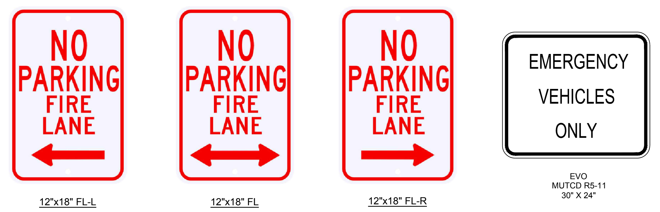
4 SIGNAGE AND STRIPING DETAILS NO SCALE NOTE: FIRE LANE SIGNS SHALL BE RED PRINT ON WHITE
