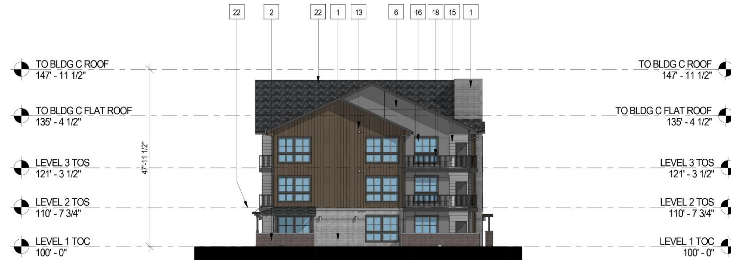
4 BUILDING C - SIDE ELEVATION 1/16" = 1'-0"
