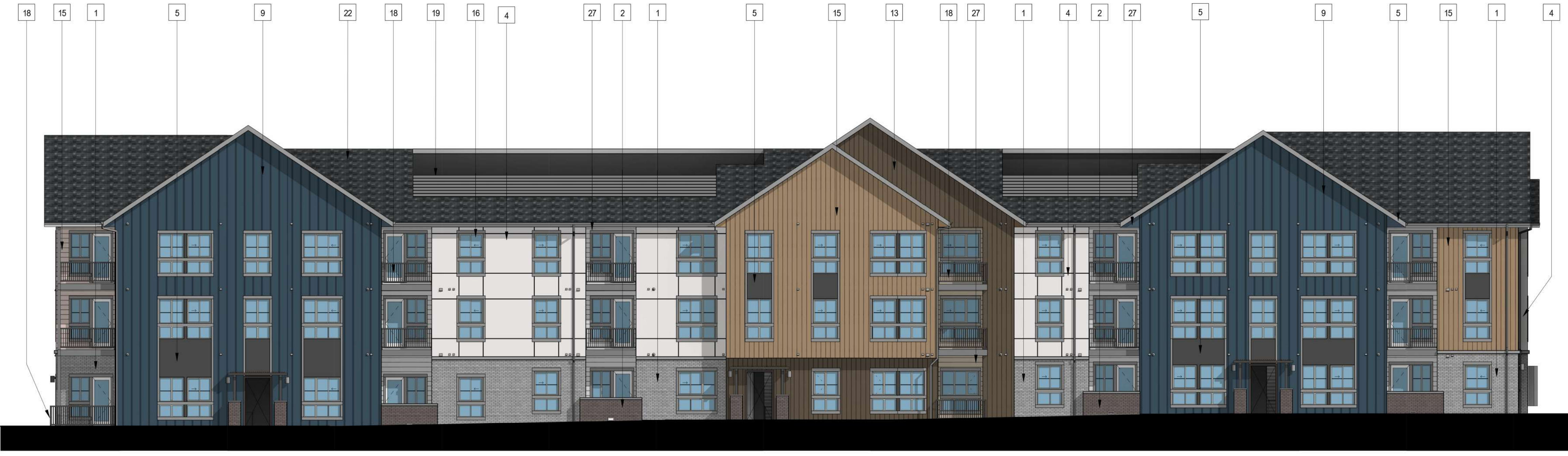
FRONT ELEVATION Note: Trim around windows shall be minimum of three and one-half (3-1/2) inches wide, and trim around doors shall be a minimum of (2) inches wide.
