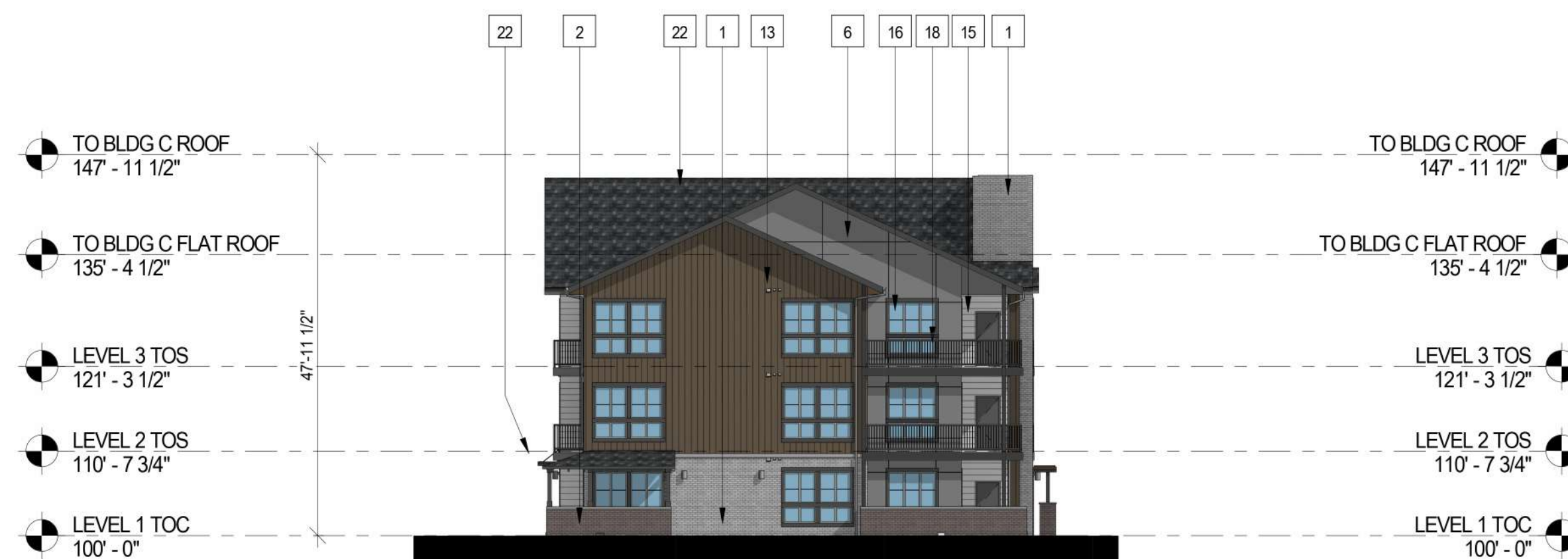
4 BUILDING C - SIDE ELEVATION 1/16" = 1'-0"
