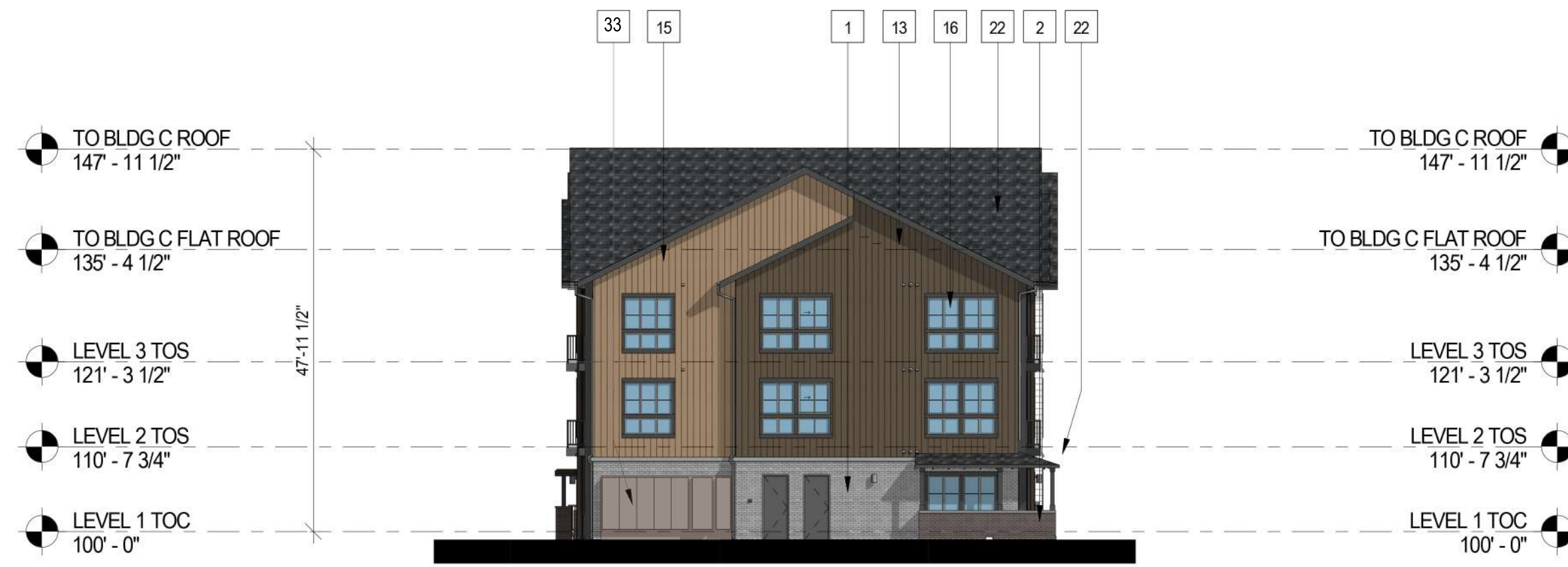
3 BUILDING C - SIDE ELEVATION 1/16" = 1'-0"
