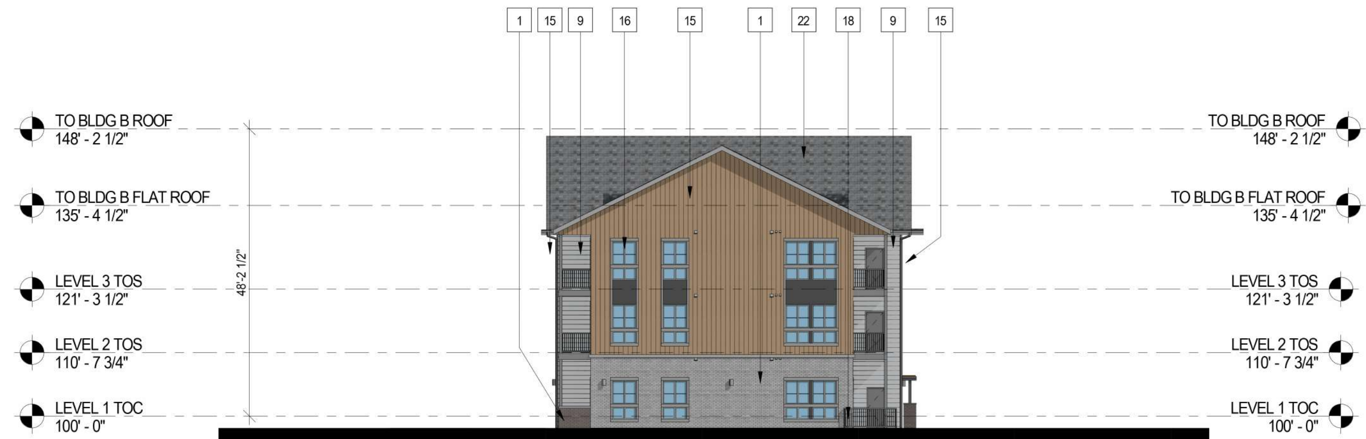
4 BUILDING B - SIDE ELEVATION 1/16" = 1'-0"
