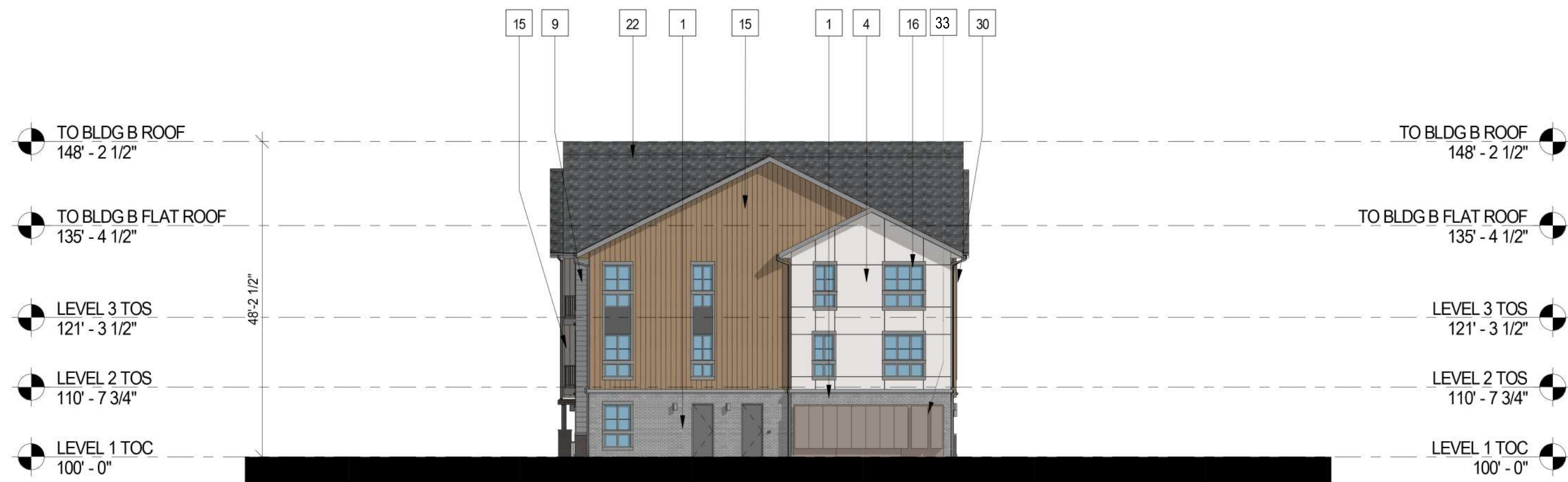
3 BUILDING B - SIDE ELEVATION 1/16" = 1'-0"
