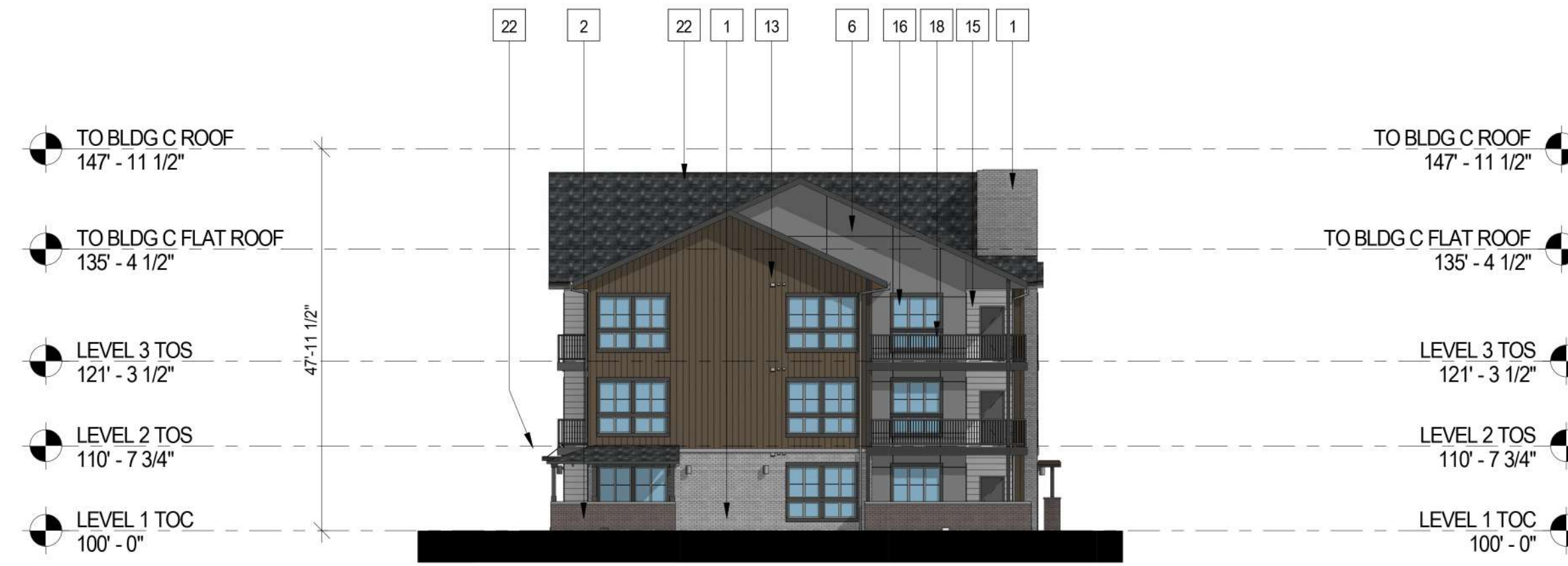
4 BUILDING C - SIDE ELEVATION 1/16" = 1'-0"
