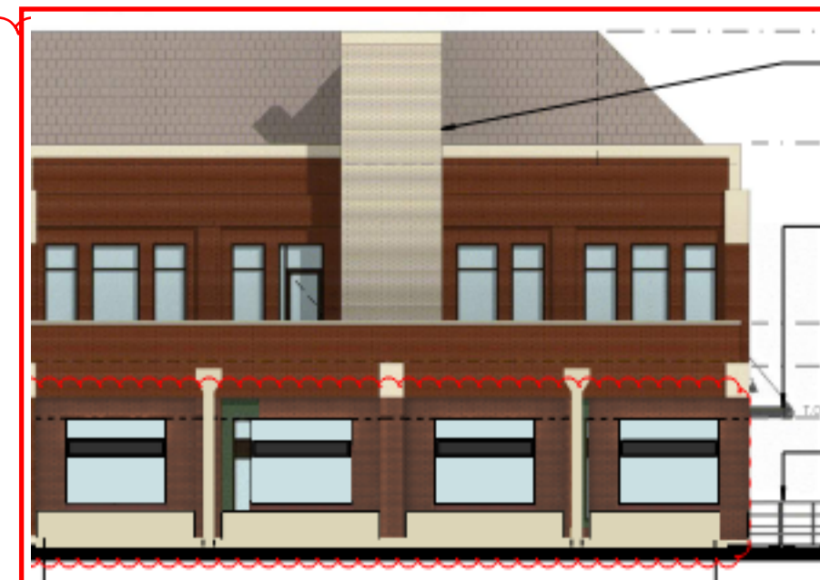
ENCLOSE EXISTING CAR DRIVE THRU WITH NEW BRICK FACADE ENCLOSURE WALL AND STOREFRONT GLAZING INFILL PANELS
