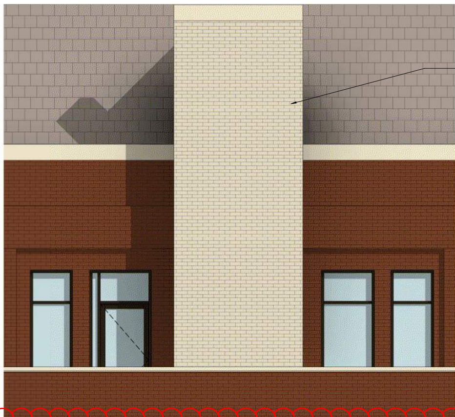
NEW BRICK MECHANICAL VENT SURROUND, HEBRON BRICK, CHAMPAGNE VELOUR
