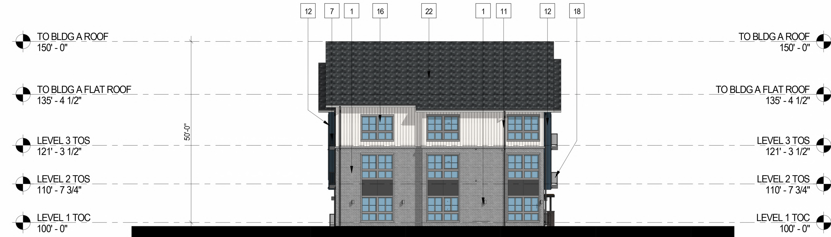
4 BUILDING A - SIDE ELEVATION 1/16" = 1'-0"
