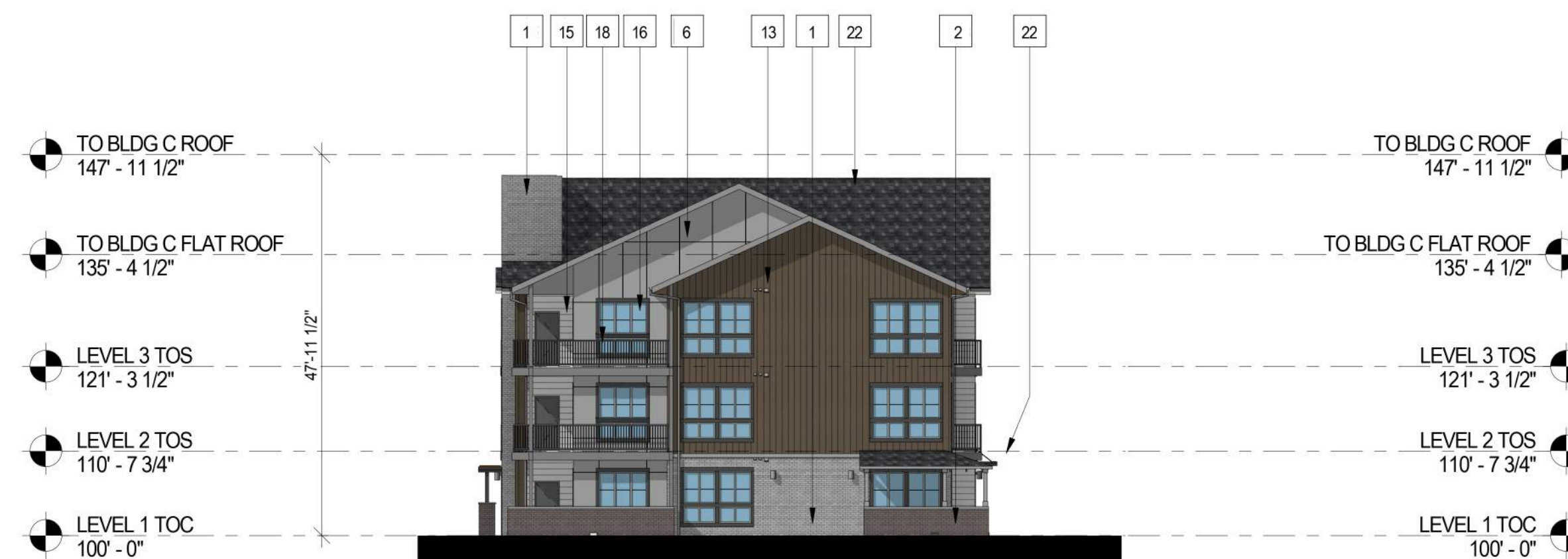
4 BUILDING C - SIDE ELEVATION 1/16" = 1'-0"
