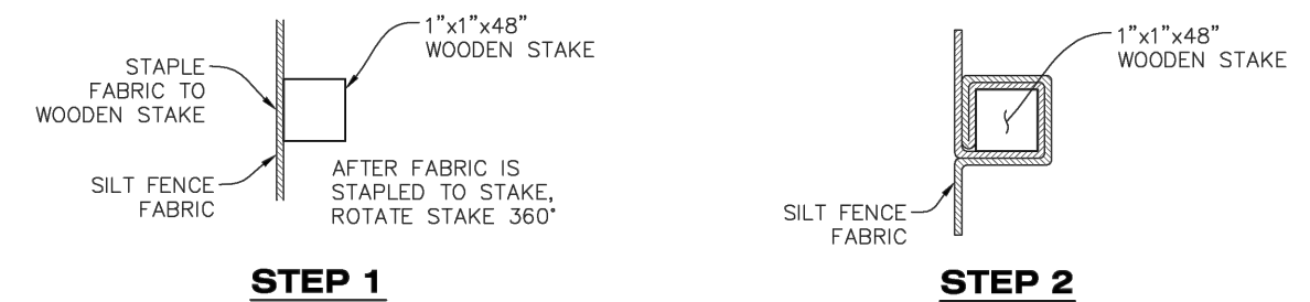
ALTERNATIVE INSTALLATION - 360° TWIST
