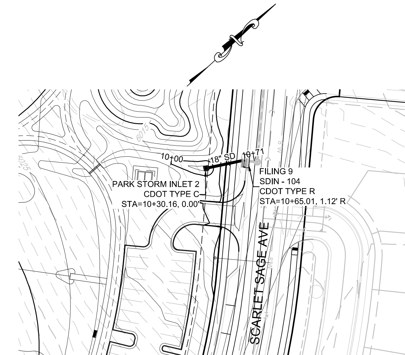
PLAN: PARK STORM LATERAL 2 HORIZONTAL SCALE: 1" = 50'
