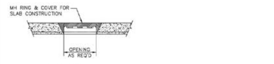
SECTION (NON-ADJUSTABLE RING & COVER TO BE CAST IN FLAT TOP) ALTERNATE RING & COVER (TO BE USED ONLY WHEN SPECIFICALLY AUTHORIZED.)
