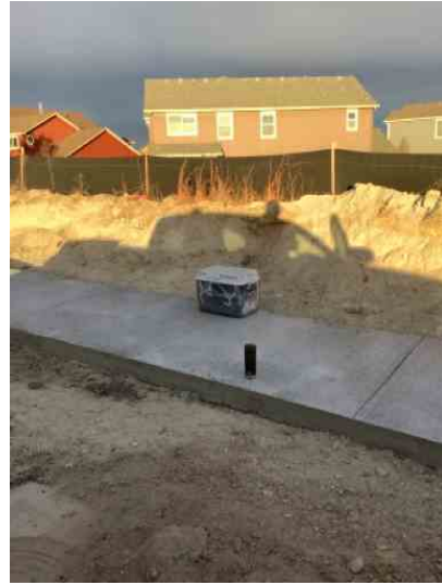
Location of cylinder samples opposite the ADA Ramp
