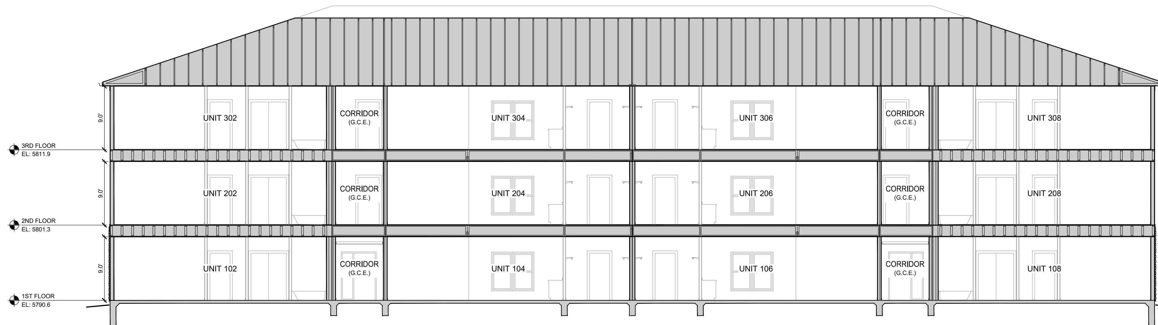
1 BUILDING 1 SECTION SCALE: 1/8" = 1'-0"
