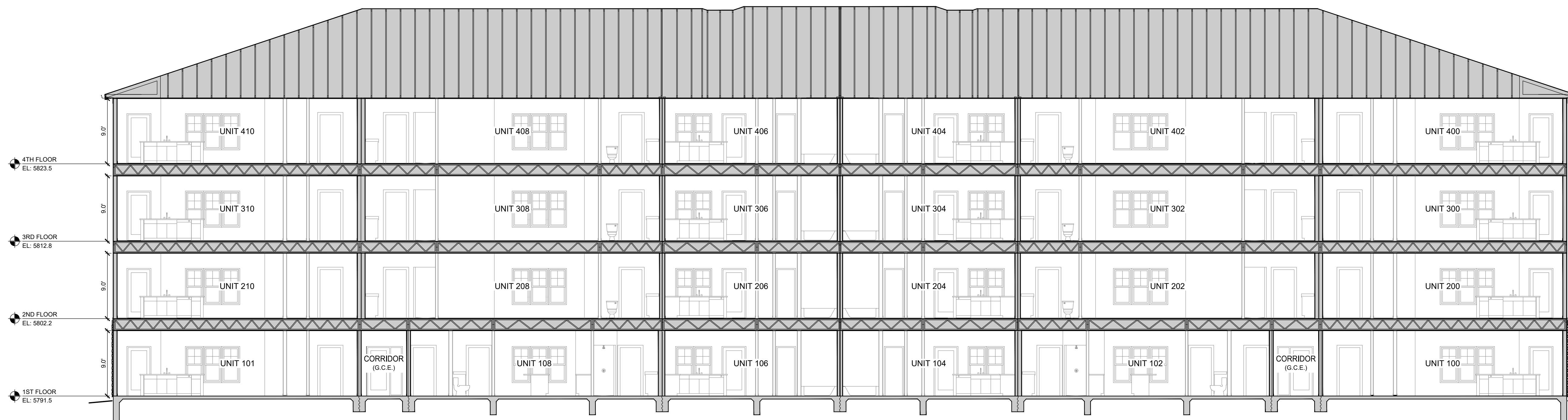
2 BUILDING 2 SECTION SCALE: 1/8" = 1'-0"
