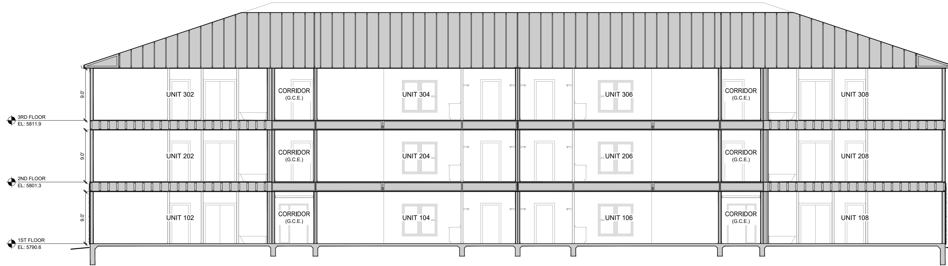
1 BUILDING 1 SECTION SCALE: 1/8" = 1'-0"
