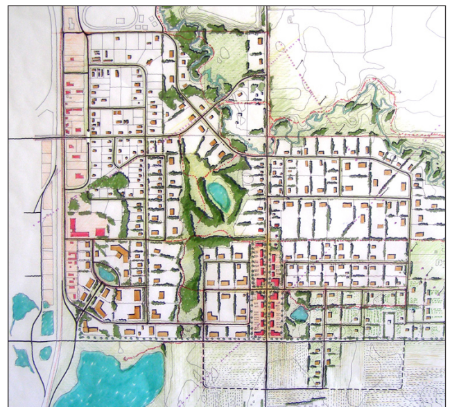
Natural features such as wetlands and creeks not only function as natural habitat and manage stormwater, but can also act as recreation amenities within a development.
