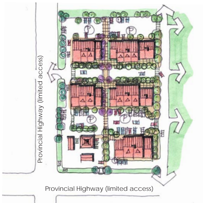
Illustration demonstrating the use of internal subdivision roads and site planning that respects the highway while still providing a welcoming commercial development
