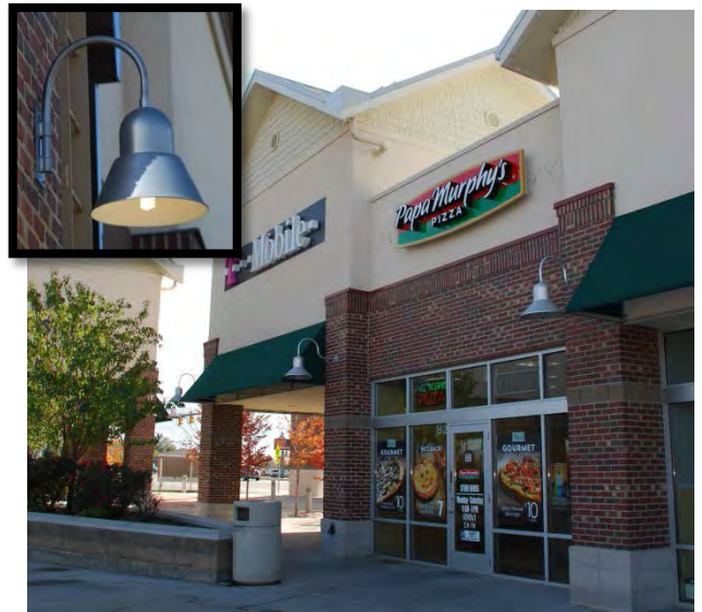
Down facing fixtures minimize light pollution
